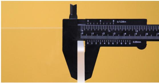
A. Heavy-gauge .25" panels for durability and stability
